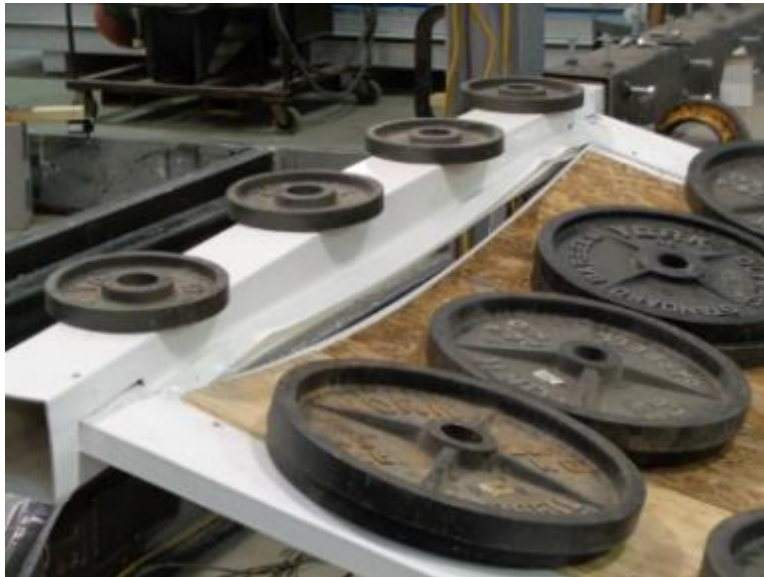
Photo No. 4 Typical Disengagement at 1.5x Design Load
